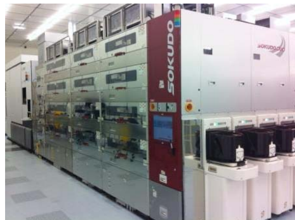
ASML NXT:1950i in-line with SOKUDO DUO lithography track inside IMEC 300mm clean room
