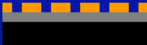
Etch hardmask and strip second resist
