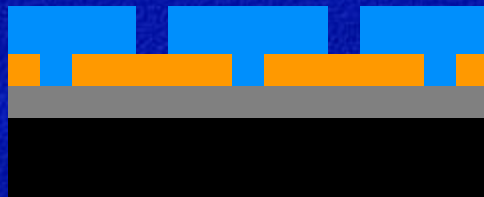
Strip first resist and coat and expose second resist
