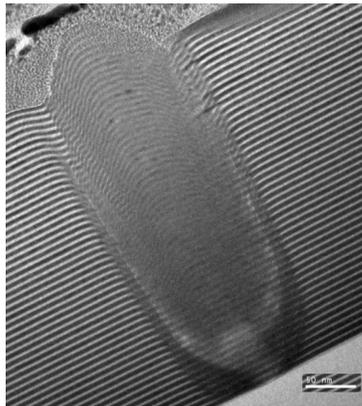
Blank defect caused by substrate bump
